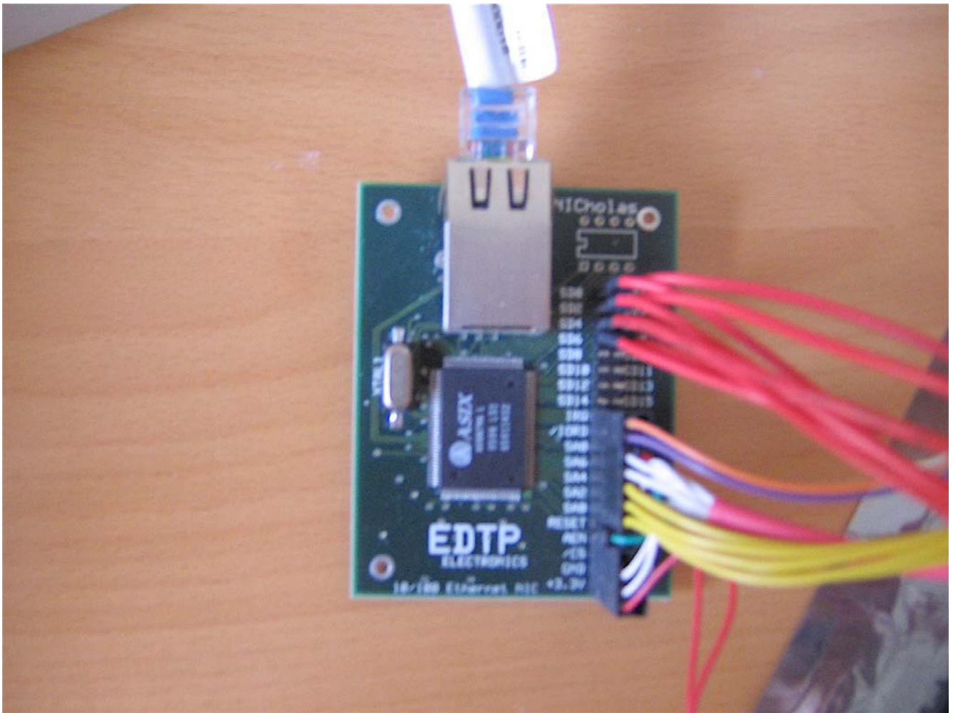
Illustration 2.: Detail of the EDTP NICHolas network interface.
